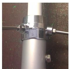
Thread in the three ground radials and secure with locking nuts.
