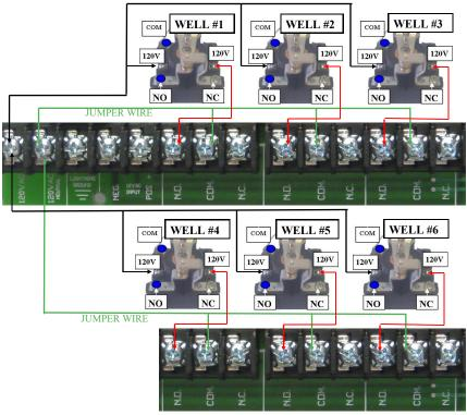
**CAUTION**: Never switch any voltage greater than 120v with the Hot Shot Receivers internal relays. This will ruin the relay and void all manufacturer warranties. Use an externally mounted 120v coil relay to switch all voltages greater than 120v. This will be shown later in Electric Well Hookup section.
