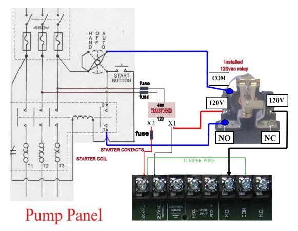
ELECTRIC WELL HOOKUP DIAGRAM W/ 3 RELAYS IN PARALLEL
