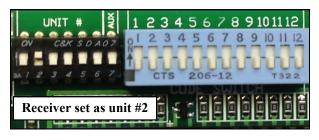
er on the transmitter you will need to use the UNIT# DIP SWITCHES located to the left of the 12-digit code bar on the receiver to program the receiver so it can be controlled by it's designated sensor ON-OFF Input on the transmitter. You can make it a #2 receiver (which is controlled by a #2 sensor transmitter) by only turning on the #2 dipswitch. See picture. You can make it a #3 receiver (which is controlled by the #3 sensor on the transmitter) by only turning on the #3 dipswitch. This
