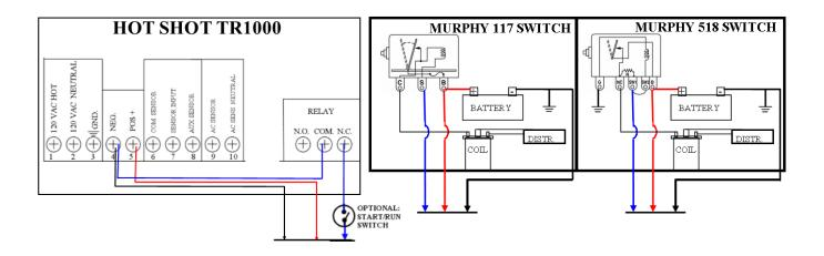
PUMP START: IF USING A START/RUN SWITCH FLIP IT TO START. POWER UP THE HOT SHOT AND START THE ENGINE AT THE PUMP. WHEN THE PIVOT IS PRESSURED UP IT'S HOT SHOT WILLTRANSMITT A RELAY ON COMMAND TO THE HOT SHOT AT THE PUMP. WHEN A RELAY ON COMMAND IS RECEIVED THE HOT SHOT WILL CLOSE ITS N.O. TO COM CONTACTS AND LIGHT UP THE RELAY LED. THIS WILL REMOVE THE GROUND FROM THE MURPHY ALLOWING THE ENGINE TO STAY RUNNING. IF USING A START/RUN SWITCH FLIP IT TO RUN.
